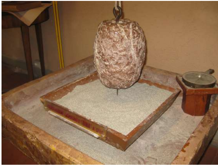
1751 Bina (Italy) simple pendulum above tray of sand
